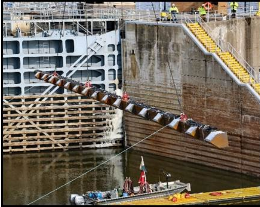
Figure 2. Photograph of the uADS speaker soundbar during deployment at Lock 19 (Photograph by Mark Cornish, USACE).
