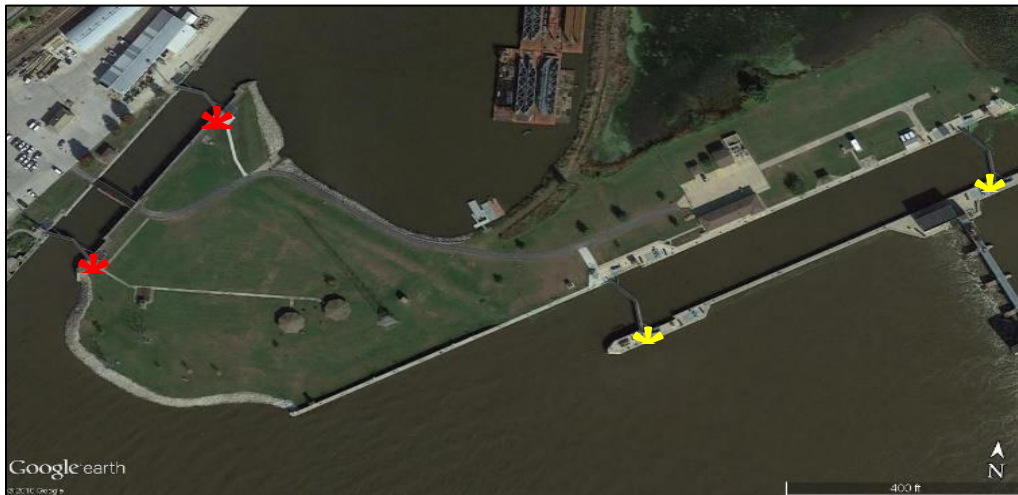
Figure 1. Locations where stationary ARIS imagery was collected in the main chamber (yellow) and auxiliary chamber (red) of Lock 14 of the UMR.
