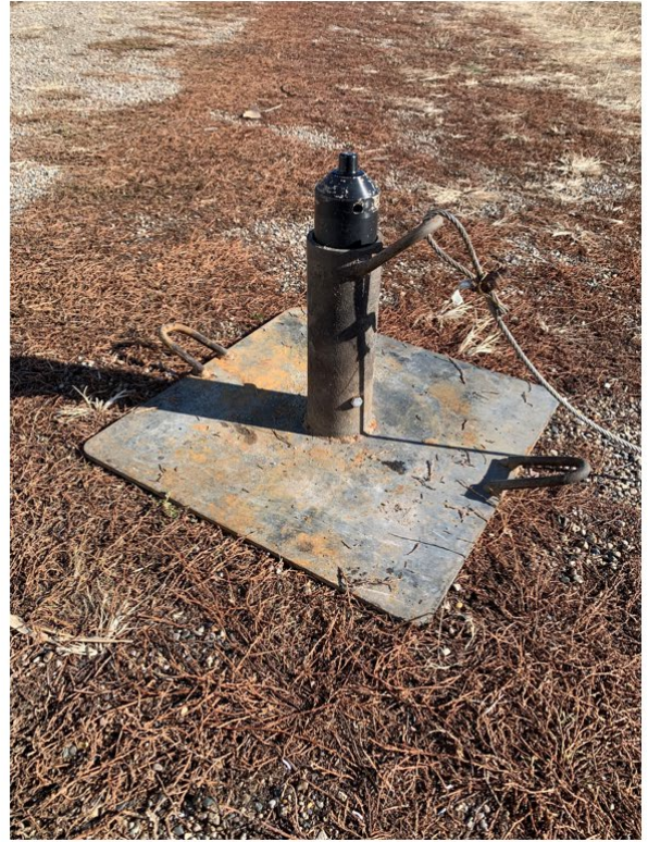
Figure 2. We deployed 19 acoustic receivers in PVC housings attached to the downstream side of intersecting highway bridges (left) and 9 bottom sets (right) throughout the study area (see Figure 1 for receiver locations). Bridge mounted receivers were oriented in a downward position and were placed at various areas of the water column depending on each site whereas bottom set receivers were pointed in an upright position approximately 0.5 m above the stream/lake bed. Bottom set receivers were anchored to the nearest shoreline with 6.5 mm cable.
