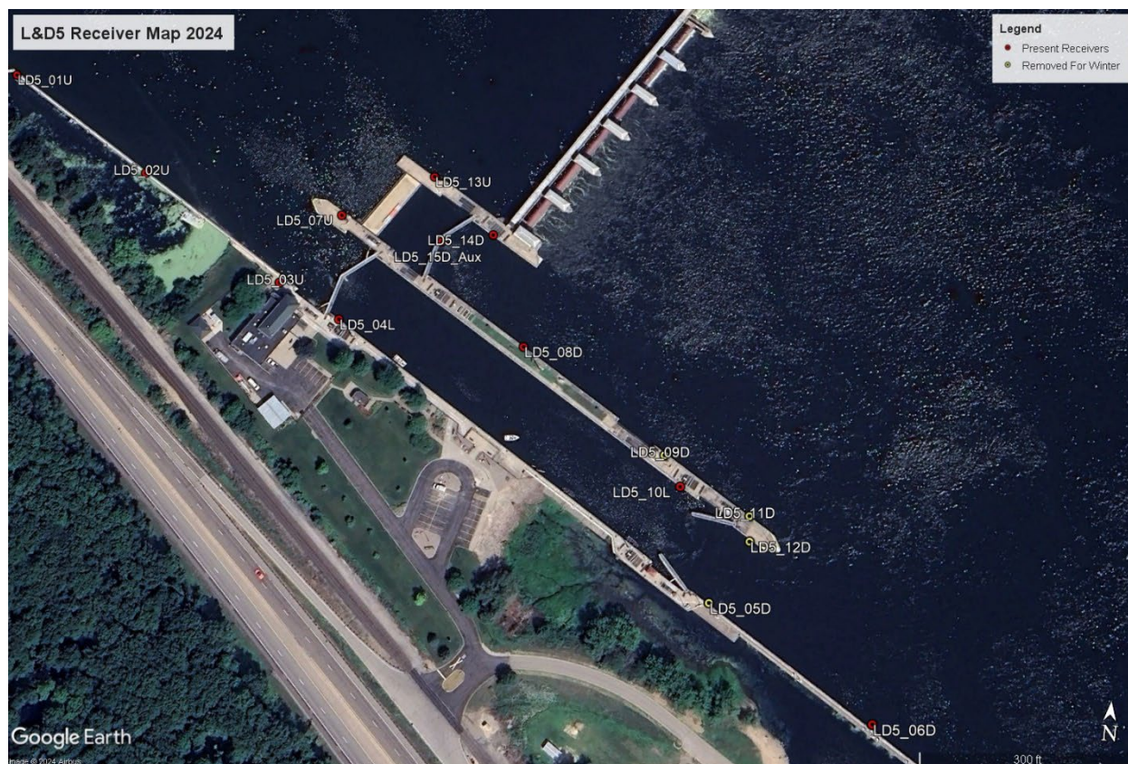
Figure 3. The 69-kHz telemetry arrays at Lock and Dam (LD) 5 in Minnesota City, MN. The receiver locations are displayed and provide coverage of the downstream lock approach, lock chamber, upstream lock approach, and areas overlooking the tailwaters and headwaters of LD 5.
