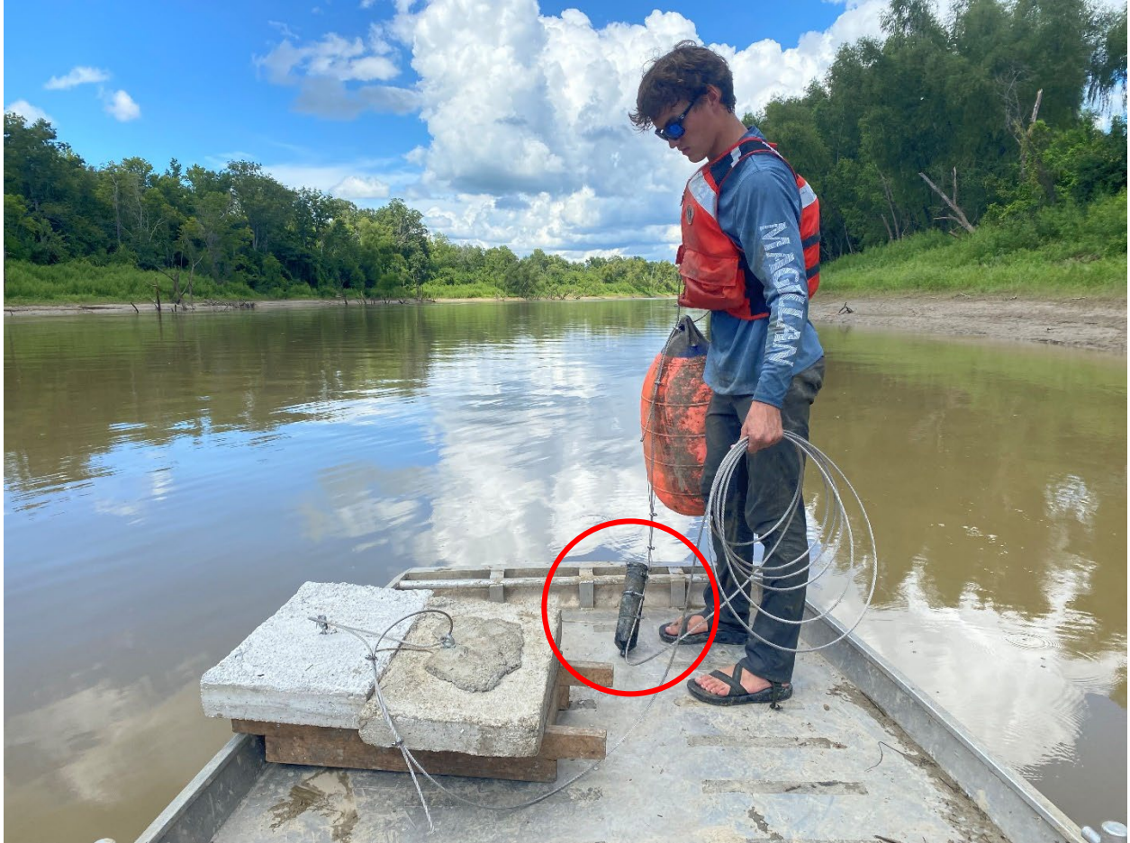
Figure 2. – Receiver (VR2) deployment. The receiver (circled in red) is attached to the large cable that goes between the orange buoy and cement weights. The receiver is attached 1.5–2 m below orange buoy.
