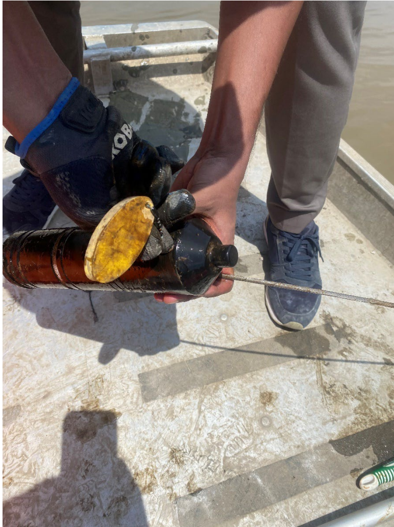
Figure 3. – Receiver with Bluetooth key inserted to initiate offload of tag detection data.
