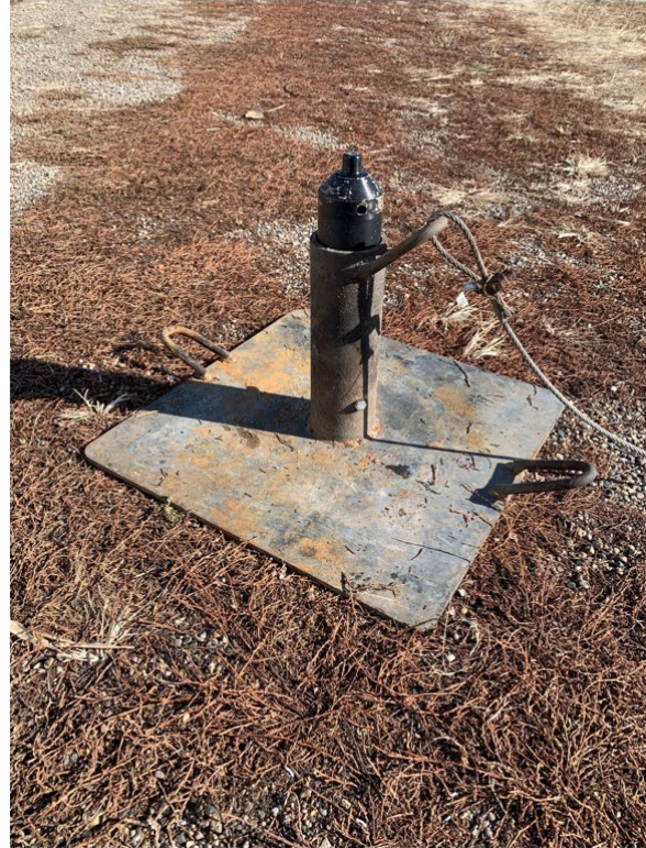
Figure 2: We deployed 19 acoustic receivers in PVC housings attached to the downstream side of intersecting highway bridges (left) and 9 bottom sets (right) throughout the study area (see Table 1, Figure 1 for receiver locations). Bridge mounted receivers were oriented in a downward position and were placed at various areas of the water column depending on each site whereas bottom set receivers were pointed in an upright position approximately 0.5 m above the stream/lake bed. Bottom set receivers were anchored to the nearest shoreline with 6.5 mm cable.
