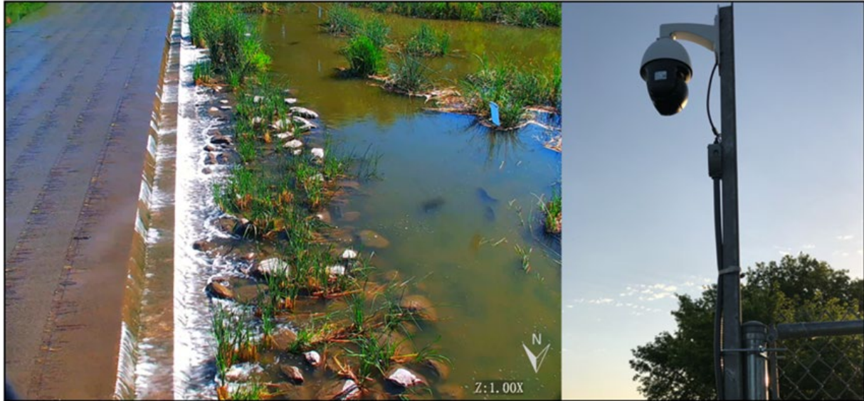
Figure 10. Outdoor video surveillance camera (Sunba network PTZ) installed above the electric fish barrier at the outlet of Lower Gar Lake on June 14th, 2022. The camera is positioned to allow for the best possible view of fish movements on the north side of the barrier.
