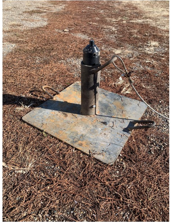
Figure 2. We deployed 19 acoustic receivers in PVC housings that were attached to the downstream side of intersecting highway bridges (left) and 9 bottom sets (right) throughout the study area (see Figure 1 for receiver locations). Bridge mounted receivers were oriented in a downward position and were placed at various areas of the water column depending on each site, whereas bottom set receivers were pointed in an upright position approximately 0.5 m above the stream/lake bed. Bottom receivers were anchored to the nearest shoreline with approximately 6.5 mm cable.
