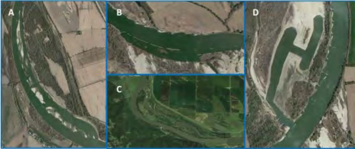
Figure 11. Habitat restoration sites in the Missouri River below Gavins Point Dam. Deer Island (A) located near Tekamah, NE represents a top-width widening project, Lower Decatur revetment lowering (B) located near Decatur, NE, Deroin side channel (C) located near Indian Cave State Park, NE, and Glover's Point backwater complex (D) located near Sloan, IA.
