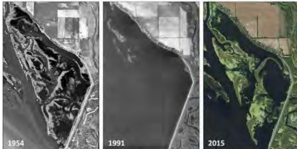
Figure 21: Restoration of habitat at Spring Lake, near Buffalo City, WI, is one example of the type of management actions implemented under authority of the Upper Mississippi River Restoration Program. Impoundment of the Mississippi River in the 1930's created many islands within the floodplain (1954). Over time, the islands eroded away, resulting in a loss of habitat quality for a variety of fish species (1991). Islands were constructed in 2005-2006 with sediments dredged from within a 600-acre backwater to restore habitat for a variety of fish species (2015).
