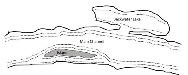
**Figure 2.** Example of survey transects (represented by dotted lines) in the Upper Mississippi River; nearshore and offshore transects for each bank along the main channel, transducers pointing toward the thalweg; one transect on each bank for island side-channels and one or more transects for backwater lakes, depending on size and bathymetry.
