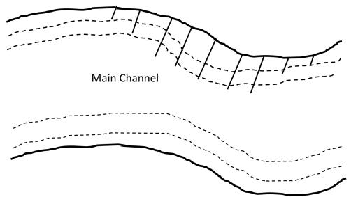
**Figure 3.** Example of main channel survey transects (represented by dotted lines) in the Upper Mississippi River where wing dikes are present. Two transects for each bank along the main channel, transducers pointing toward the thalweg. When possible, transects run over the top of the dikes and as close to shore as depth allows.
