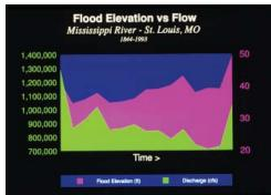
Flood elevation vs discharge (flow) at St. Louis, MO 1844 to 1993. Source: U.S. Army Corps of Engineers
