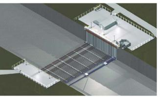
Diagram of the aquatic nuisance species (ANS) barrier located in the connecting canals between Lake Michigan and the Illinois River. Electric cables laid along the channel bed create an underwater electrical field designed to repel fish.
