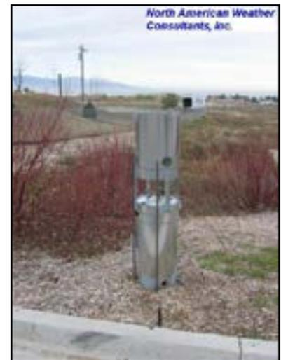
**Example of a ground based cloud nucleating generator. A propane flame is used to vaporize the seeding solution, which is composed of silver iodide mixed in acetone. The vaporized silver iodide then re-crystallizes in the cold air, forming millions of tiny particles which are intended to serve as ice nuclei. The generators are positioned to maximize the number of silver iodide crystals that reach the critical regions of passing storms. [North American Weather Consultants, Inc. Photo.](#)**
