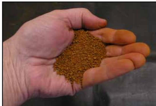
**Dry AMD sludge used for phosphorous removal from wastewater - Philip Sibrell, USGS Photo.**
